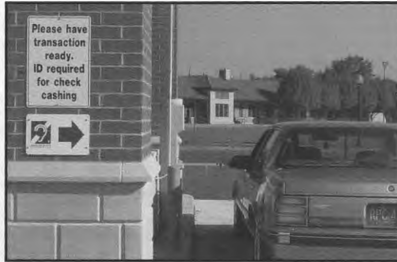
Figure 10-4: driver making bank transaction at drive-up teller window can see signage indicating loop capability and thereby can switch hearing aid from “M” to “T” for clearer reception
