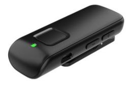
The Remote Plus can stream for up to 10 hourse on a full charge and requires 3 hours to fully recharge. An LED status indicator will blink red accommpanied by an audible tone in your hearing aids every 5 minutes when the battlery is low. The Remote Plus can be found online for anywhere from \$375.00 to \$545.00
