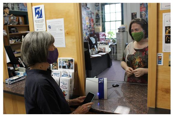
At a kiosk, cashier counter, or reception desk, the personal hearing loop can be positioned behind glass or Plexiglas, but should be as close to the telecoil user as possible. An auxiliary, plug-in microphone can pick up the staff person's voice if more sound is needed than is provided by the unit's internal microphone or if the loop is placed on the telecoil user's side of the barrier.
